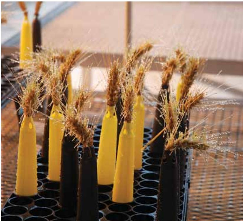
If you want to study falling numbers, you've got to study sprout, and doing that requires an apparatus which initiates the process. The wheat head mister seen here is located in the wheat greenhouse on the Washington State University campus.
